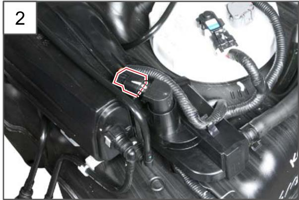
2. Disconnect the canister shut off valve connector on the top of the air filter of the removed fuel tank assembly. (KOREA)
